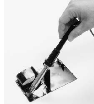
An alternative to the hotplate crackle test is using a soldering iron and glass test tube.
