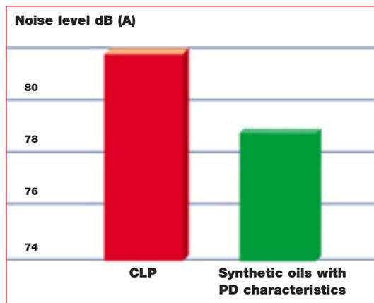
**Smoother surfaces and lower temperatures reduce the noise of gear units**
