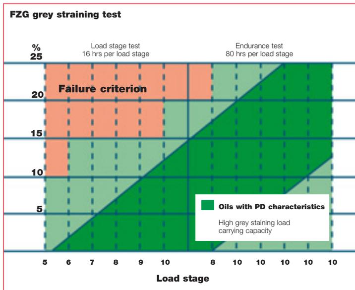
**Test procedure for grey staining load carrying capacity**
