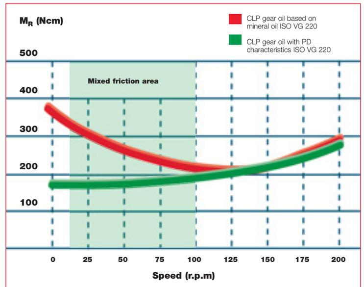
**The PD additives immediately form an anti-friction protective layer in the contact area**
