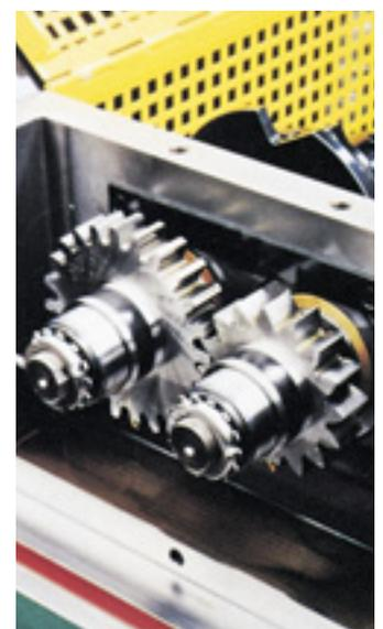
**Test gear of the FZG test rig**
