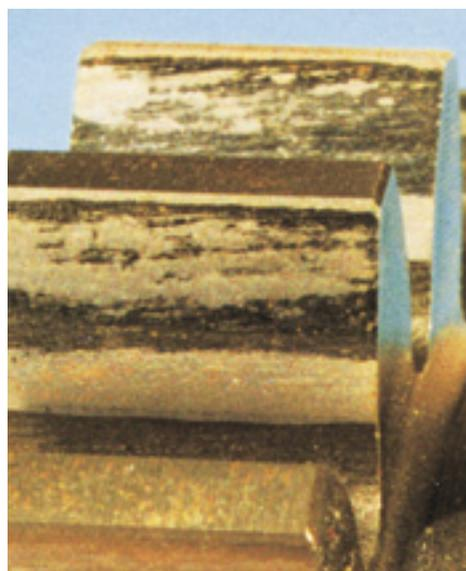
**Grey staining is fatigue damage that results from insufficient lubricating film or excessively high sliding speed**
